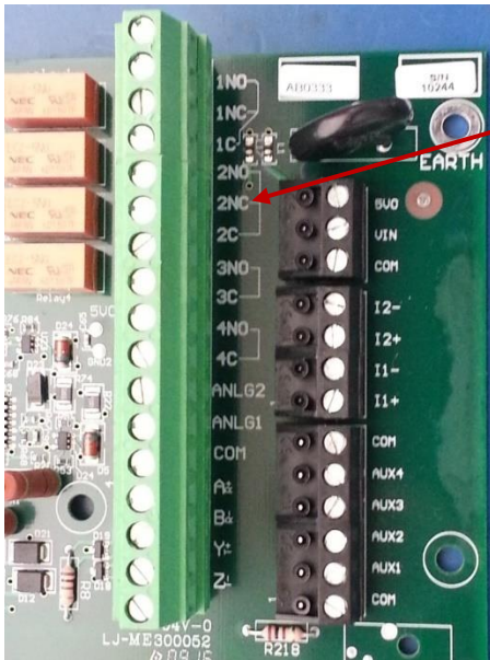
Figure 24 – Programmable Relays for Lead/Lag Control
