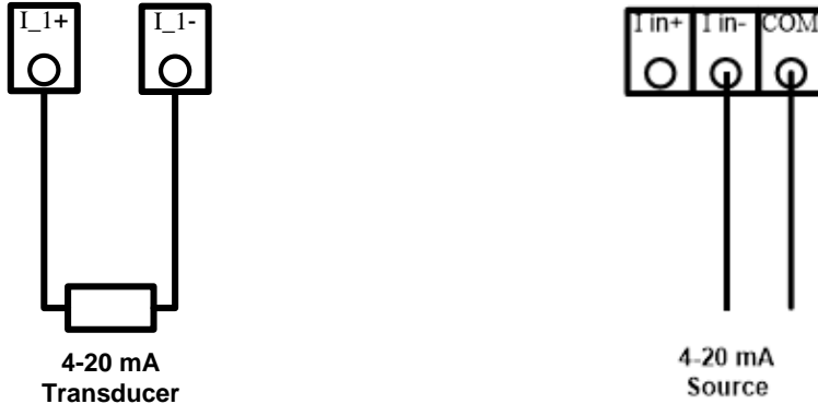
a. 4-20 mA Transducer Connection
